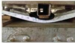
Roof Tile TBS 002 Tile at maximum deflection of 20mm
