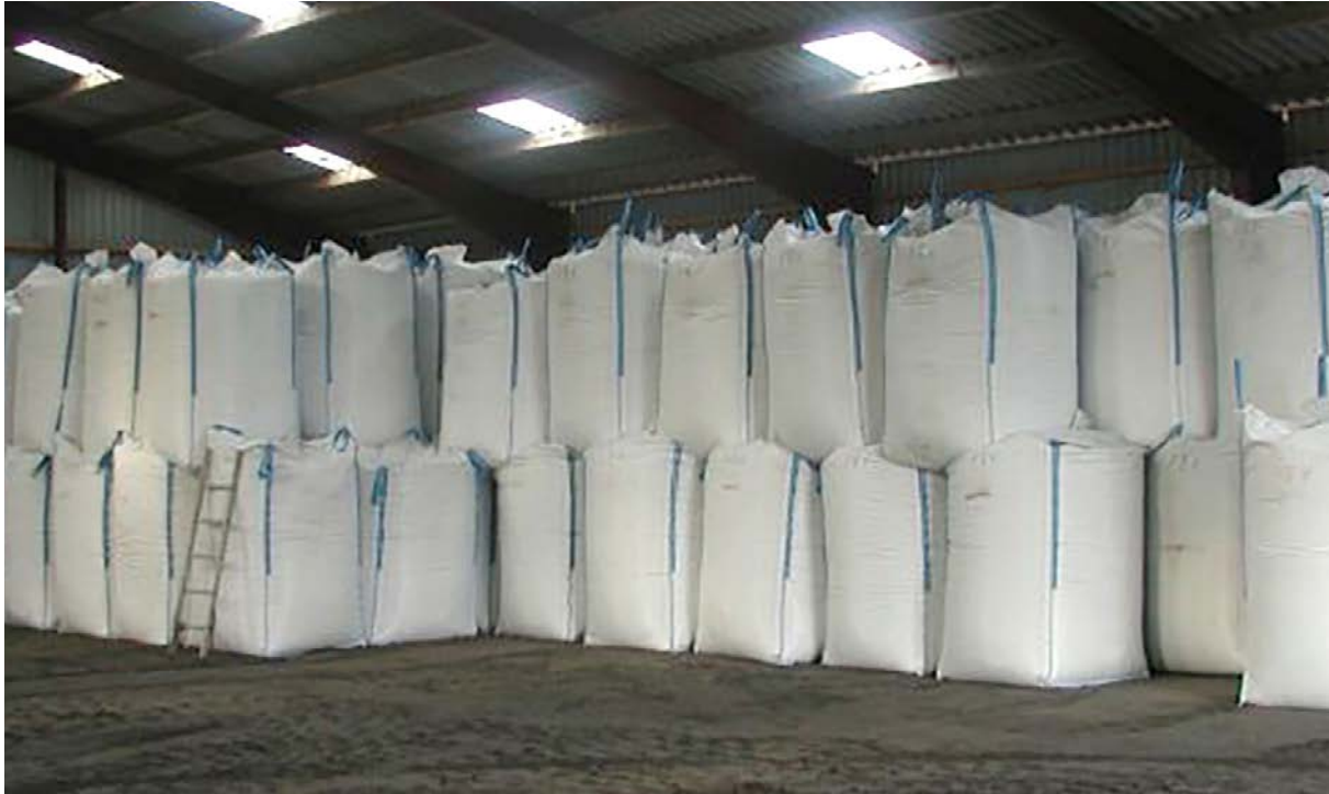
Air pollution control residues in big bags from an incineration plant in Denmark awaiting disposal. These neutralisation residues are normally disposed of in German saltmines. Promising new technologies will in future limit the residues to be disposed of.
